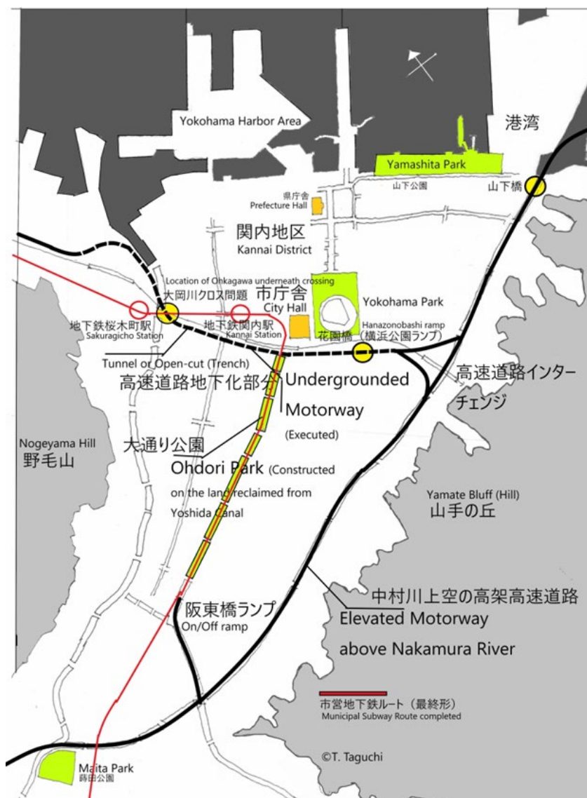
Fig.18 The finally agreed part of underground motorway (dotted line) and its connecting elevated motorways above Nakamura river. Source: own elaboration.
