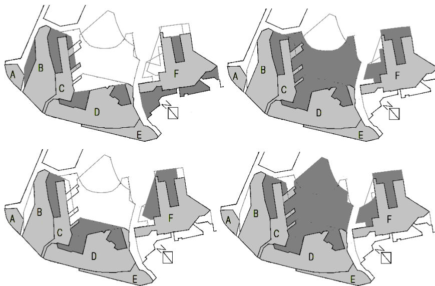
Figure 18 Different concepts of land reclamation volume required for MM21 development at different stages Legend: upper left is the original proposal by Tamura in 1964, lower left is an innovative concept by the Planning and Coordination Bureau under Tamura's directorship supported by Ohtaka architect office in 1975, upper right is the preliminary plan in 1981, and lower right is the final one in 1982.
